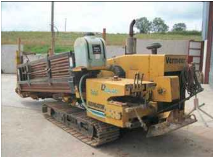
Typical Directional Drilling Rig
